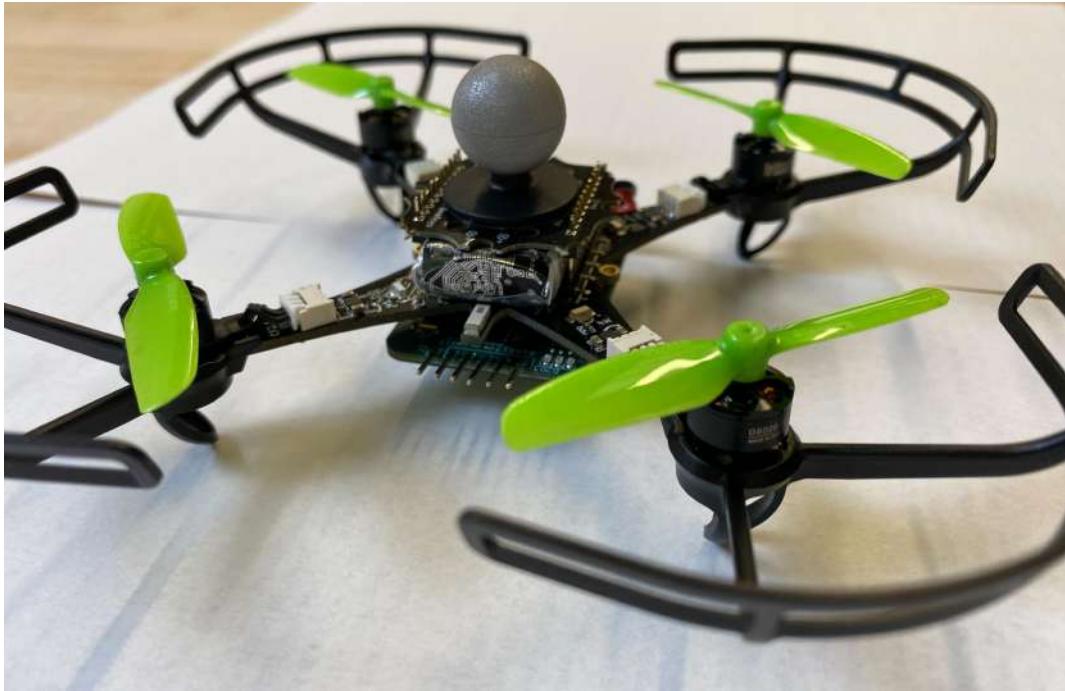
Figure 4.9: Drone with the FPGA board integrated beneath the main board and the motion capture marker mounted on top.
